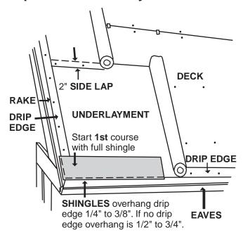
**Installation:** When applying underlayment, keep the product as wrinkle-free as possible. Unroll the underlayment parallel with the eaves. The underlayment should go over eaves' drip edge flashing, but go under the rake's drip edge flashing.
